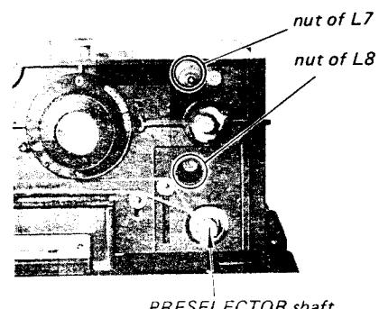
1. Turn the PRESELECTOR shaft to make the springs of L7 and L8 visible as shown on the right.
