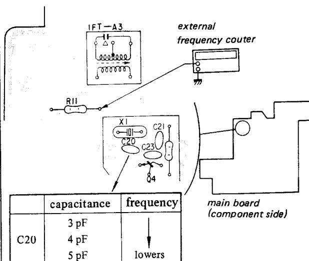
Adjust the value of C20 so that the frequency reading on the frequency counter becomes 18.6 MHz  $\pm 250$  Hz.
