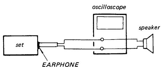
1. Set the receiver to tune in to 20.0 MHz.
